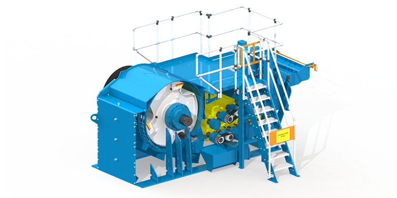
Image: The drum chipper includes a service platform, to allow for easy and safe access, and for facilitating knife change
